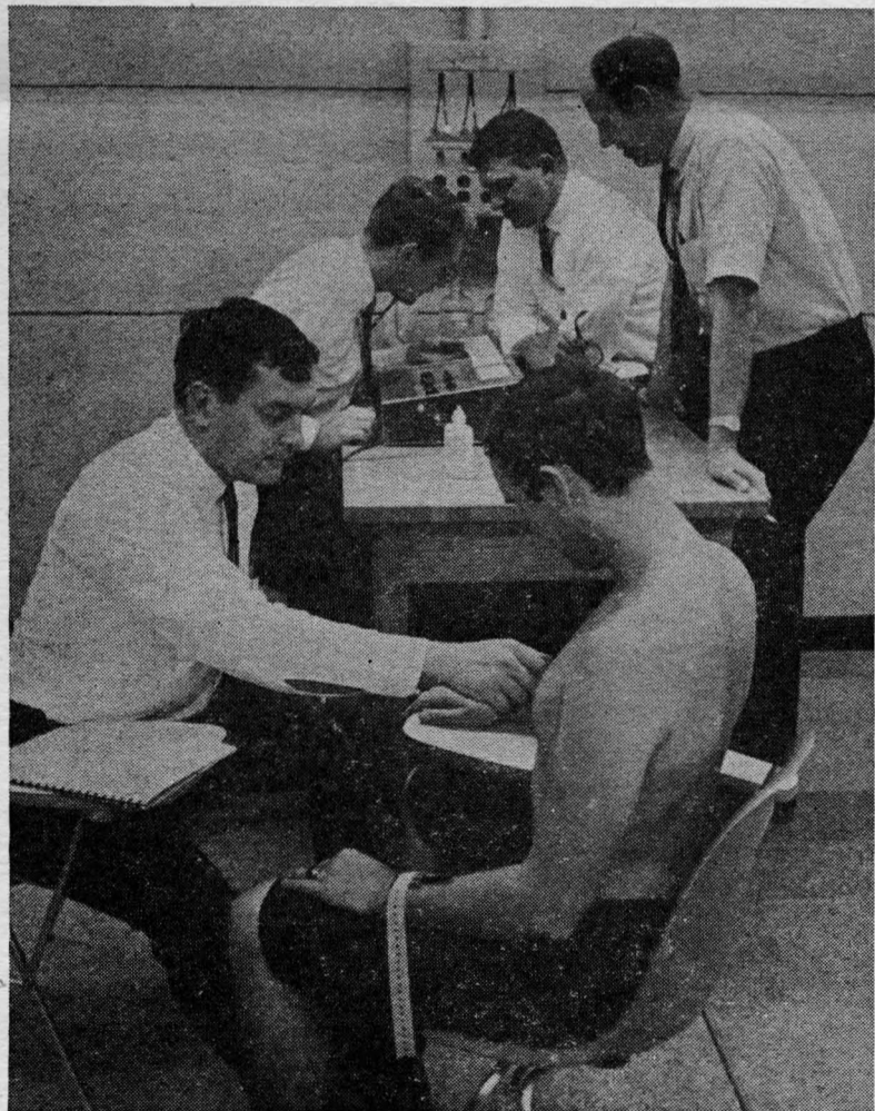
Bioengineering student Jim Lees applies electrodes to fellow student Erich Allmer to pick up minute electric potentials from the heart. In the rear instructor Ray Jefferis operates the electrocardiographic recorder as Professor N. R. Kornfield and student Ernest Purcell look on.
